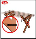
For bench construction, you will follow the same basic directions you used for the table, except that the dimensions are different. For instance, use half-inch spacers separating the two seat slats. And the crossed bench legs should be cut at 24-degree angles rather than at 38 degrees. Note that the brace will need to be offset by one-half inch to accommodate the space between the slats.
