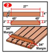
Using a combination countersink bit, drill two screw holes into the cleat above each slat, deep enough to set the screw heads below the surface. Fasten to the slats with 4" screws.
