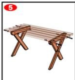
6. a Mark and cut the table braces to fit between the table leg assembly and the table top with 45-degree angles at both ends.
